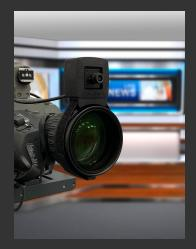
LiveView is an option for the TR-XT control system and uses a simple miniature HD camera mounted on the robotic-controlled full broadcast camera to provide the LiveView scene. The TR-XT touch screen enables the operator to select any area of the LiveView scene to control the main camera's motion.
