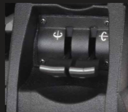
Pan and tilt brake controls
