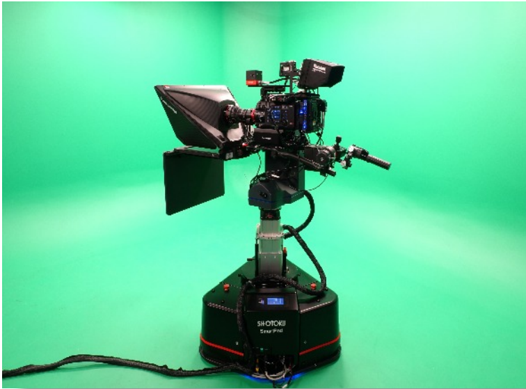
ANS - SmartPed with external third-party VR/AR tracking camera
